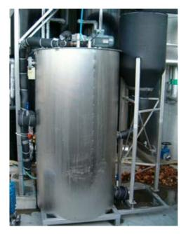
Figure 10: Anaerobic bioreactor<sup>1</sup>.
