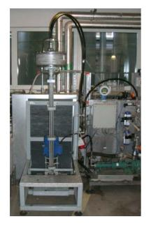
Figure 11: VSEP unit (membrane stack and electrical engine)<sup>1</sup>.
