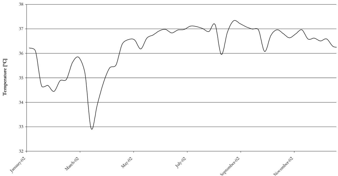
**Figure 4. Temperature variation in all anaerobic digesters during 2002. The temperature is a mean value of the temperatures in all anaerobic digesters over the period.**
