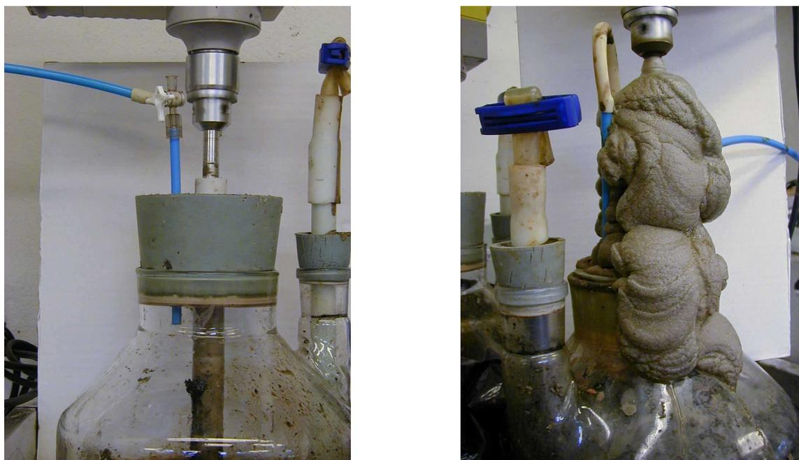
**Figure 23. Two experimental reactors from the laboratory at the Tekniska Verken in Linköping for the development of the process aid KMB1. The left-hand photograph shows the experimental reactor with KMB1 added and the right-hand photograph shows the reference reactor. The photographs were taken on the same day; while the experiment was being performed with a high load.**
