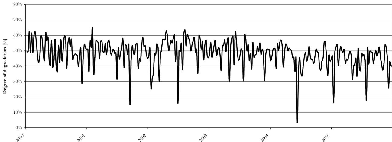
Figure 21. Degree of degradation of the organic matter during the evaluation period, calculated with Formula 8.
