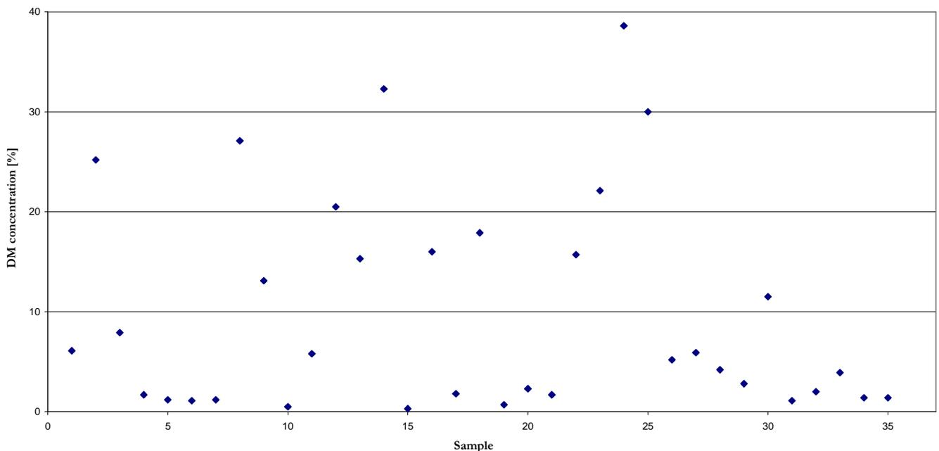
Figure 15. Analysis of the concentration of the DM [%] in grease separator sludge.
