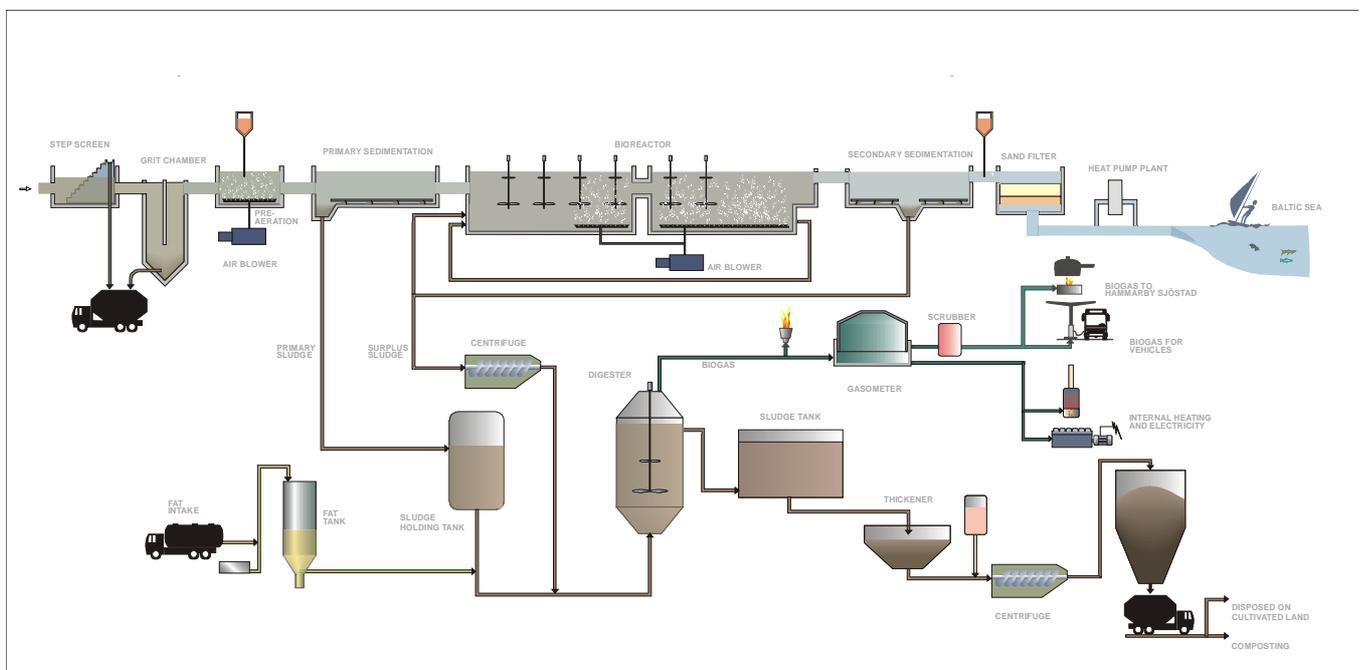
Figure 1. Overview of the wastewater treatment process at Henriksdal. The diagram has been obtained and modified on the basis of information material belonging to Stockholm Water Company AB<sup>1</sup>.
