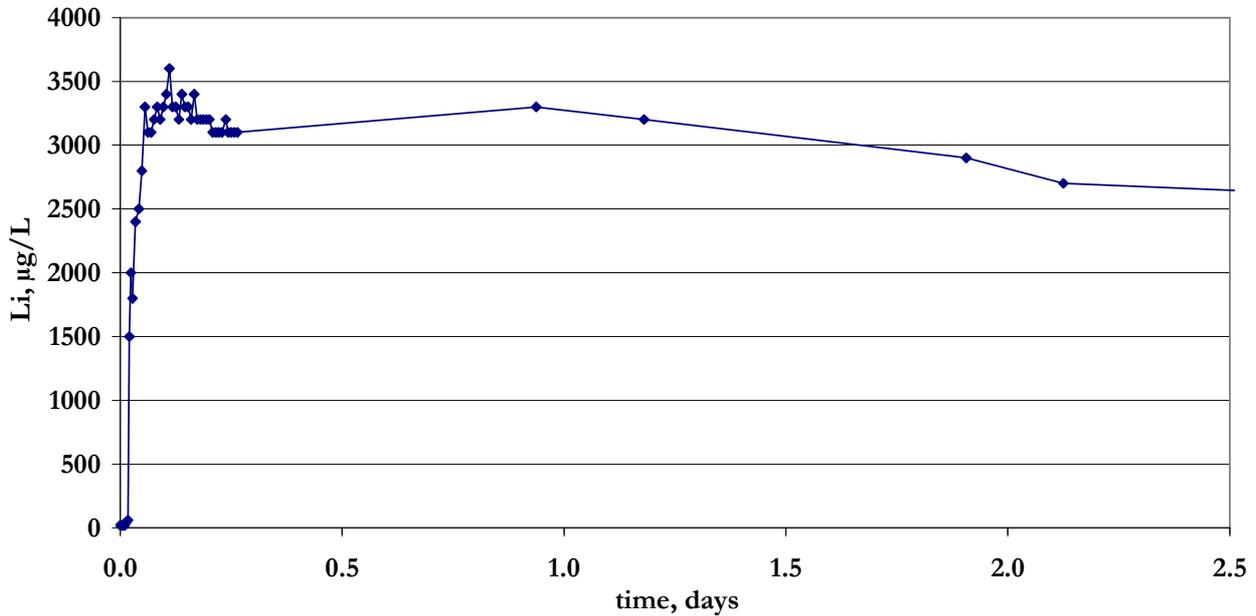
Figure 8. Li concentration in the effluent from the anaerobic digester 5 as a function of the sampling time.
