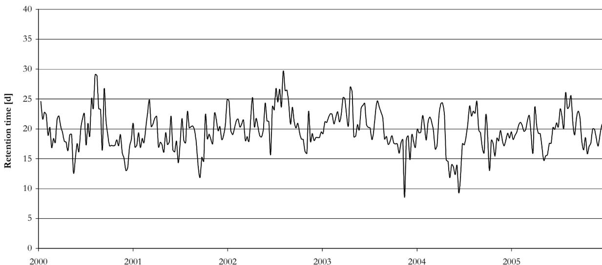
**Figure 6. The retention time in the digestion process at Henriksdal calculated from the total volume of all seven anaerobic digesters. Only the volumes of digesters in operation have been considered in the calculation of SRT.**
