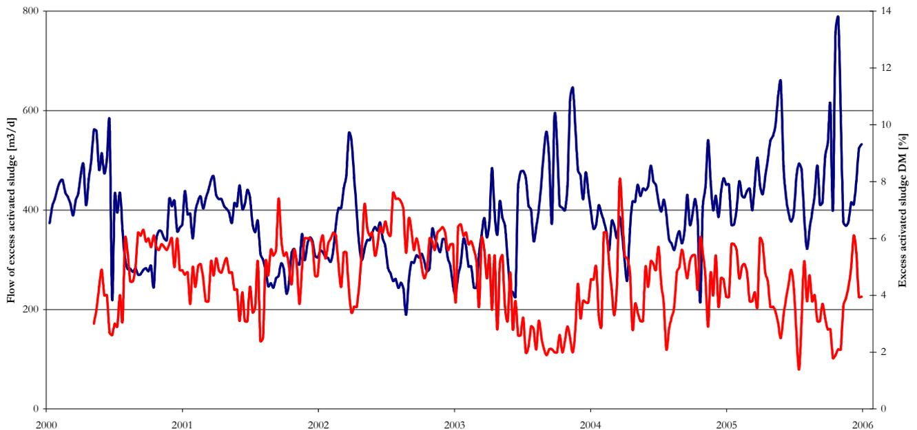
**Figure 13. Flow (—) and DM concentration (—) of thickened excess activated sludge pumped to the digestion process.**
