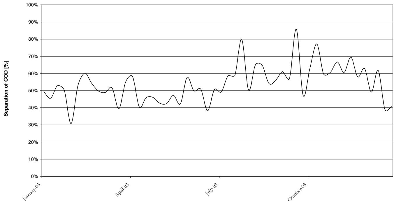
Figure 12. Separation via the pre-sedimentation process during 2003.
