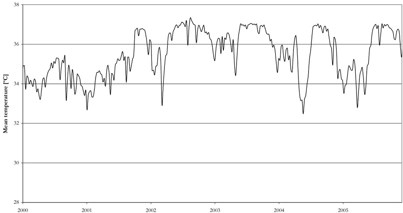
Figure 5. Mean temperature in active anaerobic digesters during the evaluation period.
