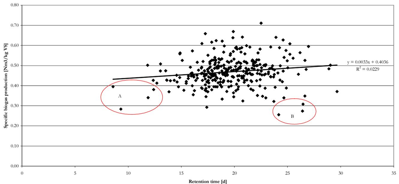
Figure 18. Specific biogas production as a function of retention time (HRT). The linear regression shows that there is no strong correlation between the variables.
