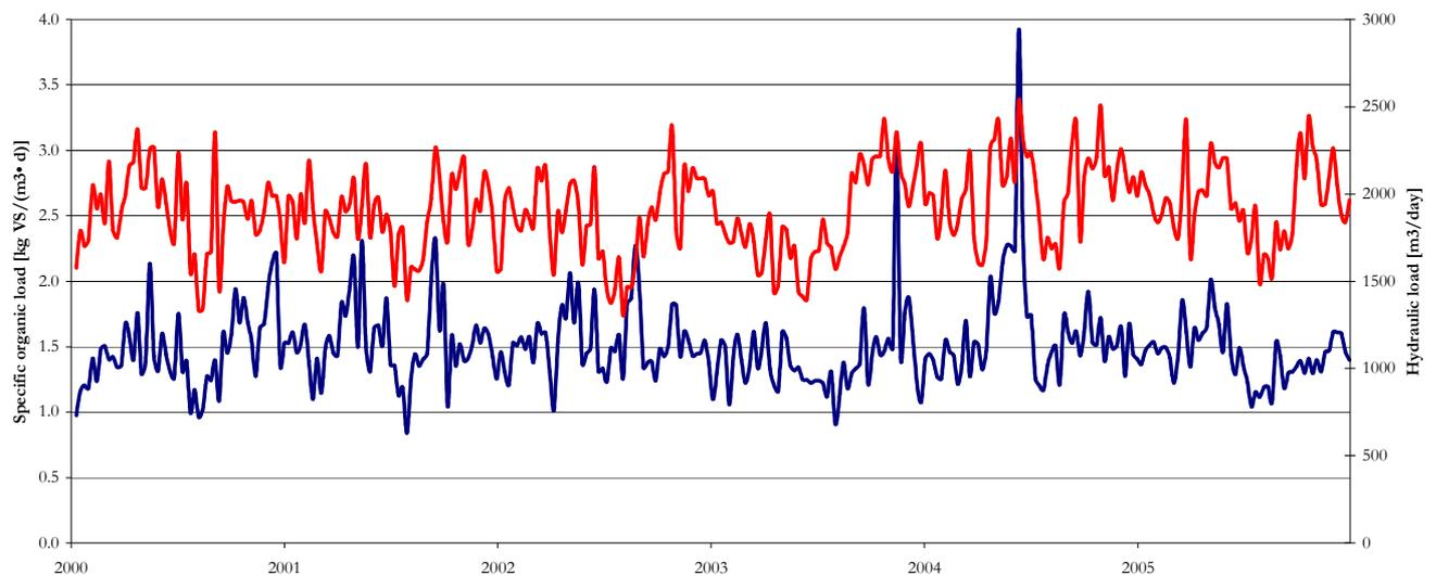
Figure 10. The specific organic load (—) and the hydraulic load (—) on the digestion tanks.
