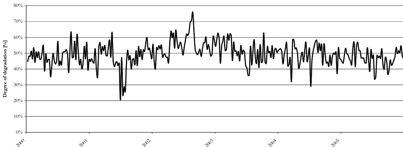
**Figure 20. Degree of degradation of the organic matter during the evaluation period, calculated with.**
