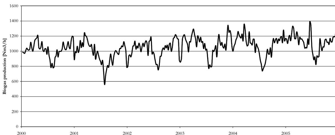
**Figure 16. Total biogas flow (Nm<sup>3</sup>/h) from the digestion process during the evaluation period.**
