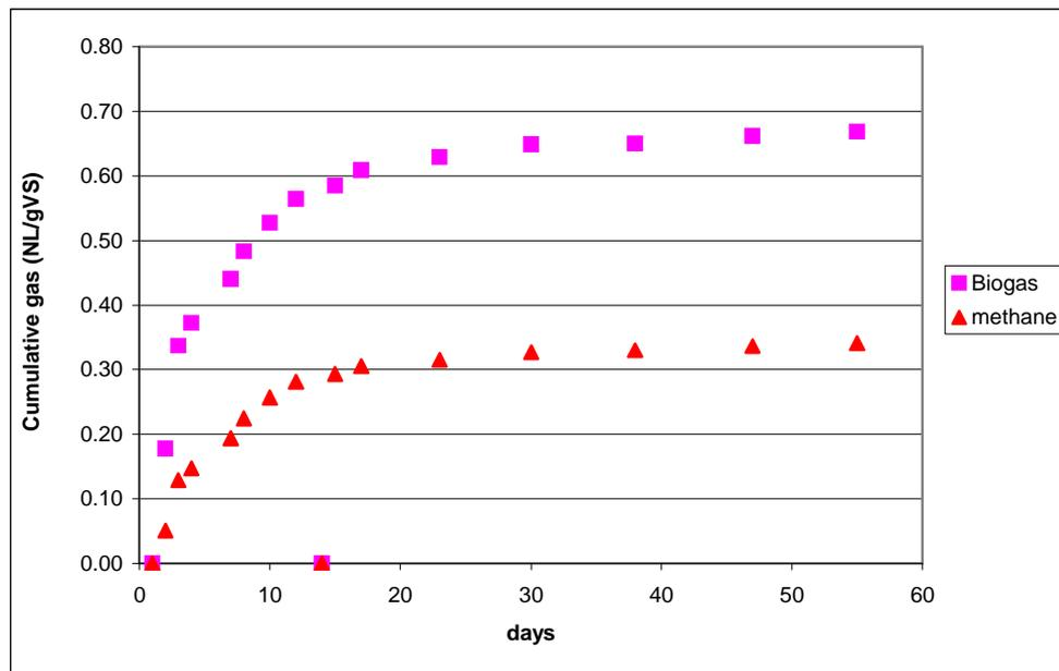
Figure 1. Cumulative biogas and methane production in relation to VS supplied from blending of primary and excess activated sludge.
