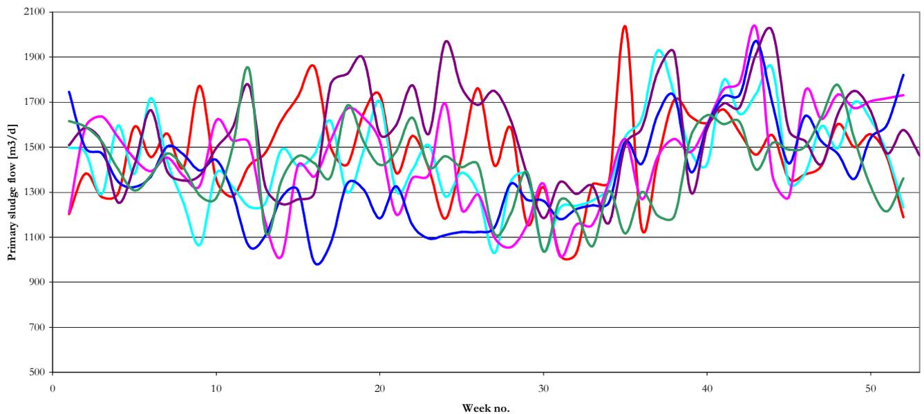
**Figure 11. Primary sludge flow for the digestion process during 2000 - 2005 varies with the season. The values are floating means for four weeks so as to identify annual variations more clearly. Years 2000 (—), 2001 (—), 2002 (—), 2003 (—), 2004 (—) and 2005 (—).**
