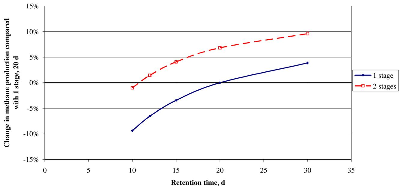
Figure 19. Expected change in methane production in serial operation compared with parallel operation in the case of a retention time of 20 d. Calculations carried out with the aid of data from JTI's digestion investigation corrected with the assumption that degradation takes place approximately twice as quickly in the case of good stirring.
