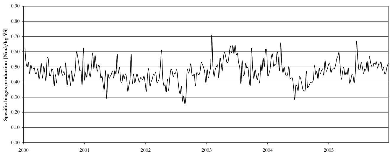
**Figure 17. Specific biogas production from the digestion process during the evaluation period.**
