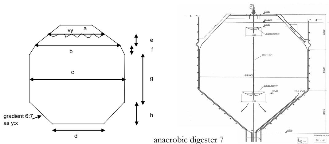
**Figure 2. Diagram of an anaerobic digester (not proportional) with dimensions according to Table 2 (on the left), and scale drawing of AD7 (on the right). The top stirrer is not included in this drawing.**
