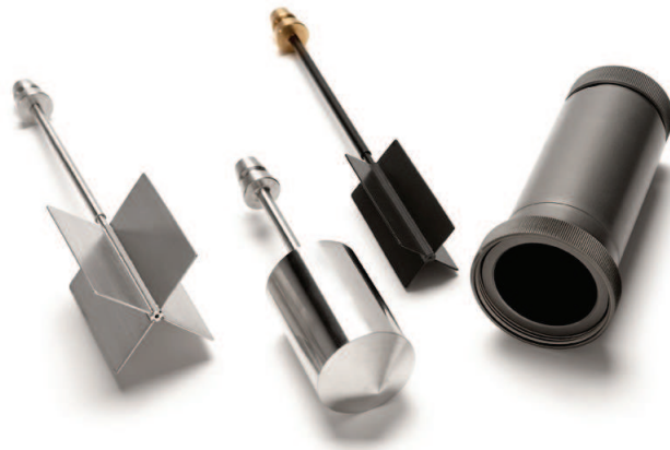
Figure 3: The different rheometer inserts (bob and vanes) and cup. N.B. the smaller vane was used here .
